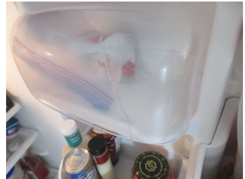
Damaged internal compartment
